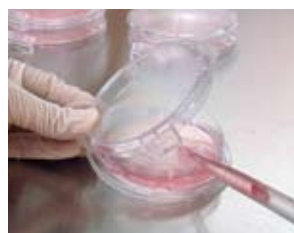
(SHellDisH) It is possible to open and close by single finger.
