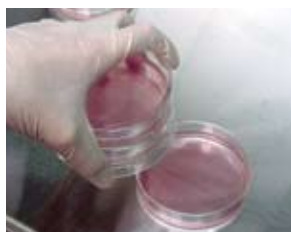
(Ordinary Dish) It has a problem that lid and basement dish will separate easily.
